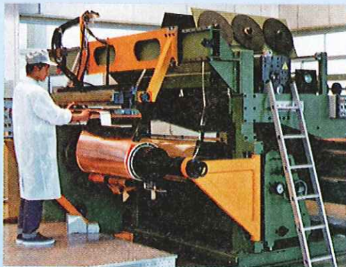
SHEET-CONDUCTOR WINDING OF A SECONDARY COIL
