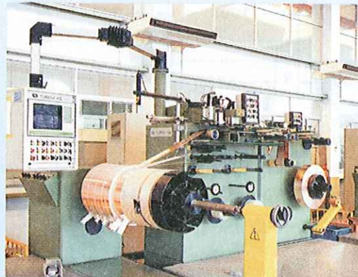
STRIP-FOIL WINDING OF A PRIMARY COIL
