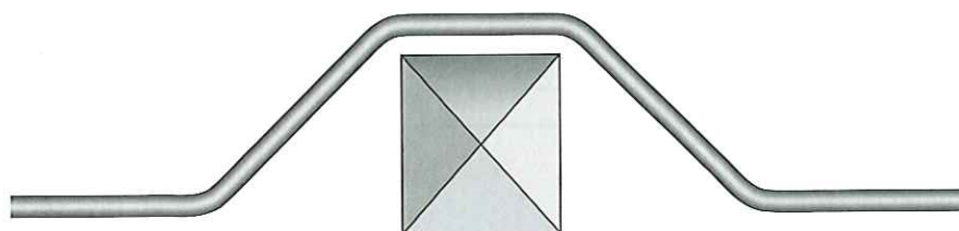
Figure 19 ♦ Typical four-bend saddle.
