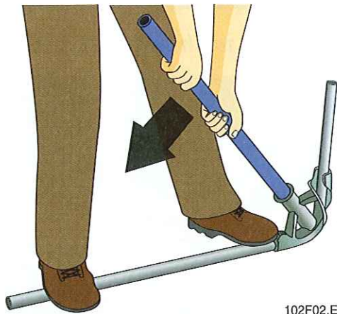
Figure 2 ♦ Pushing down on the bender to complete the bend.
