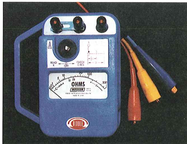
Figure 34 ♦ Earth ground resistance tester.
